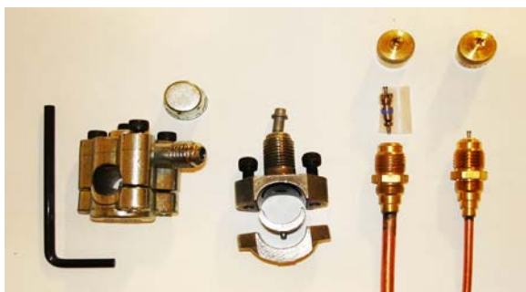
Figure 226A Piercing Valve와 Schrader Valve
